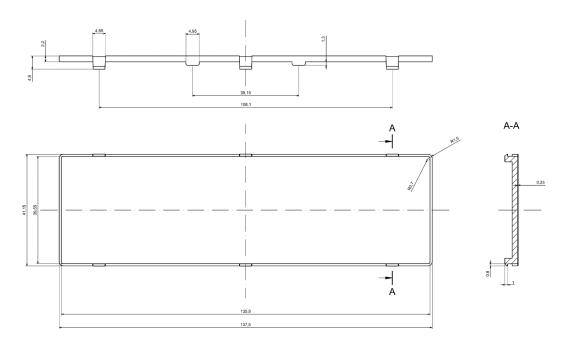
All dimensions are given within +/-0,5mm tolerance
