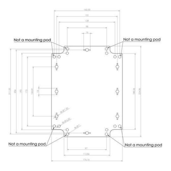
Dashed line shows outline of the mounting boss under PCB board Recommended mounting holes diameter ø4mm
