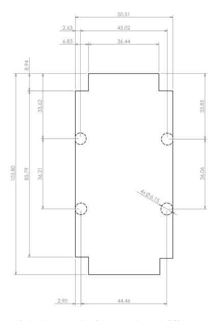
Dashed line shows outline of the mounting boss under PCB board Recommended mounting holes diameter ø3,5mm All dimensions are given within +/-0,5mm tolerance
