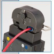
The AMT4001 (M22520/40-01) crimp tool is a fast, manually operated tool for crimping AS7928 (MIL-T-7928) Ring Terminals and Splices for wire sizes 26 through 14 (terminal and splice color codes Small-Yellow, Red, and Blue).
