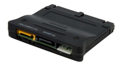
The PATA2SATA3 is a bi-directional SATA IDE adapter/converter that lets you connect a Serial ATA drive to a legacy IDE port, or an IDE drive to a SATA motherboard port.
