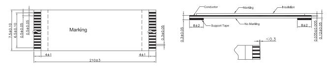
Dimensions : Millimetres Tolerances: ±0.3mm
