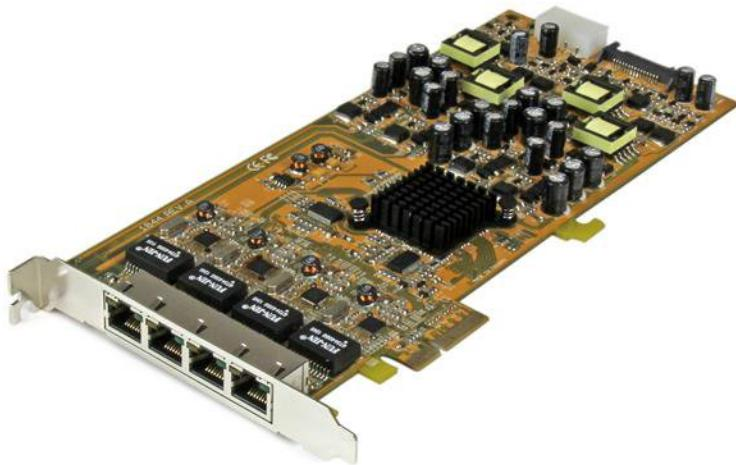
The ST4000PEXPSE 4-Port PoE NIC lets you add four Gigabit Power over Ethernet ports through a single PCIe slot. Each port can provide up to 25.5W of power, combining network data and power over a single Ethernet cable for reduced cable clutter and added convenience for remote PoE devices.
