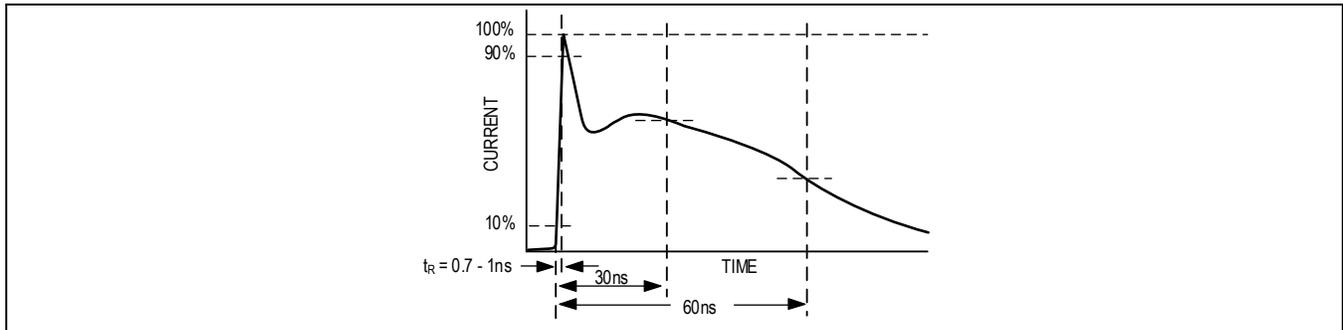
Figure 11. IEC 61000-4-2 ESD Generator Current Waveform
