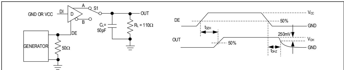
Figure 4. Driver Enable and Disable Times ( $t_{DZH}$ ,  $t_{DZH}$ )
