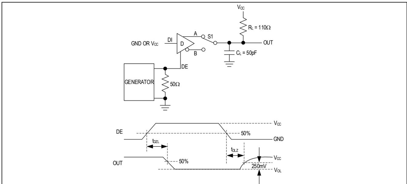
Figure 5. Driver Enable and Disable Times ( $t_{DZL}$ ,  $t_{DLZ}$ )
