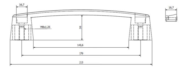
Materials: 15% Glass-filled Nylon 6; Threaded Insert CZ121 free cutting brass.
