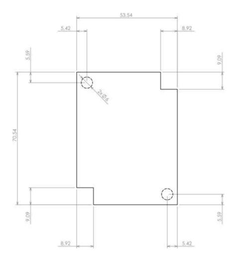
Dashed line shows outline of the mounting boss under PCB board Recommended mounting holes diameter ø3,5mm All dimensions are given within +/-0,5mm tolerance
