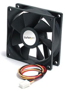
This quiet, dual ball-bearing (9.25cm) Case Fan offers a cost-effective solution for replacing a non-functional or noisy fan in your PC. Powered through a simple TX3 connection to the host computer power supply, the 8cm case fan helps keep your computer running at optimal temperatures for stable system performance.
