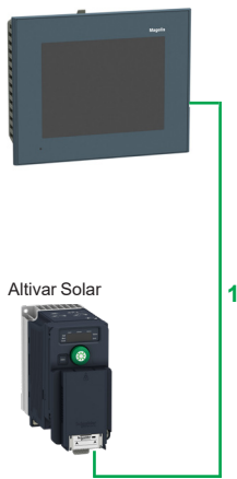
Example of connection of an Altivar Solar drive and a Harmony GTO advanced touchscreen panel via the Modbus serial link
