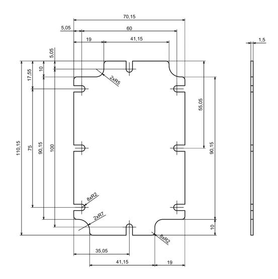
All dimensions are given within +/-0,5mm tolerance
