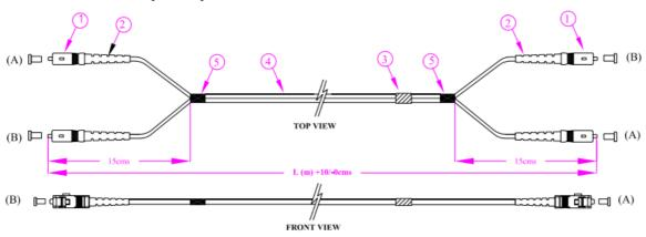
**Connector:** SC Clips shall be mounted to the connector to make it duplex.
