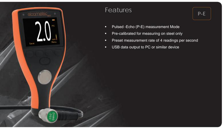
With automatic transducer recognition, which ensures correct probe identification even when the transducer is changed, a measurement rate of 4Hz (4 readings per second) and integral zero disc, ensuring maximum accuracy of  $\pm 1\%$ , the MTG2 is ideal for taking basic thickness measurements.
