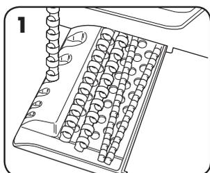
1. Select the correct comb diameter using the comb storage tray.
