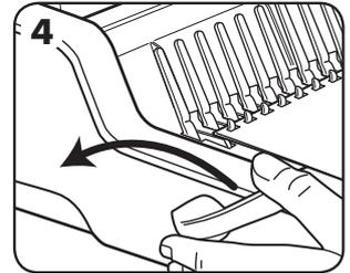
4. When all punched sheets are loaded onto the comb, push the comb lever backwards to close the comb and remove the bound document.
