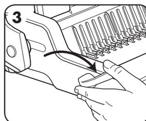
3. Pull comb-opening lever forward to open the comb.
