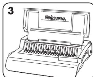
3. Lift the lid. Ensure the comb-opening lever is pushed backwards.
