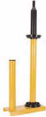
Heavy duty dispenser for pallet stretch film W400-500mm x 38/50/78mm cores
