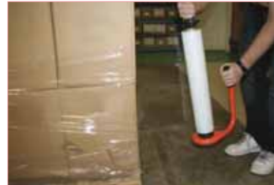
Heavy duty dispenser for pallet stretch film W400-500mm x 38/50/78mm cores
