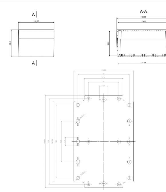
Dashed line shows outline of the mounting boss under PCB board Recommended mounting holes diameter ø4mm All dimensions are given within +/-0,5mm tolerance
