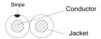
Cable Marking: RS PRO 2 Core × 0.34 mm<sup>2</sup> Speaker Cable 60V
