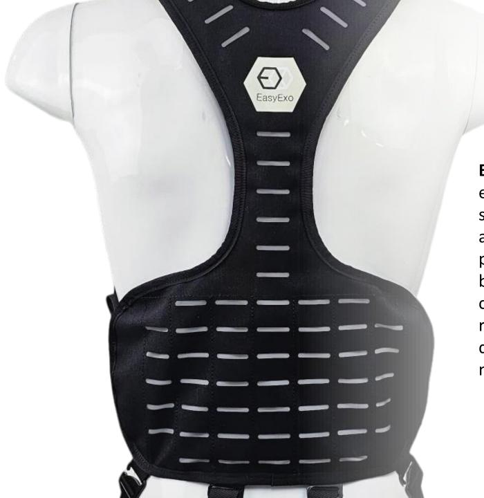
EasyExo Exoskeleton acts as extra back muscles. Elastic bands stretch during muscle extension and recoil during contraction, providing energy and assisting bending motions. They move comfortably with the user, reducing strain on spinal muscles during bending or squatting. No motors or batteries are required.
