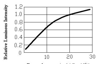
Forward current (mA) Ta=25°C Luminous Intensity vs. Forward current
