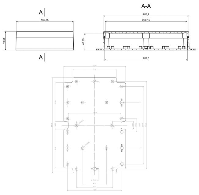
Dashed line shows outline of the mounting boss under PCB board Recommended mounting holes diameter ø4mm All dimensions are given within +/-0,5mm tolerance
