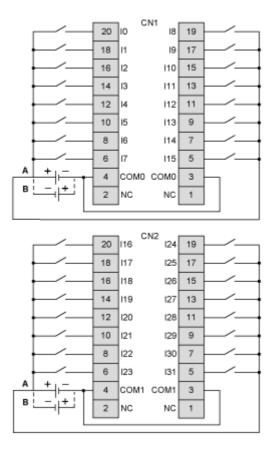
The COM0 and COM1 terminals are not connected internally
