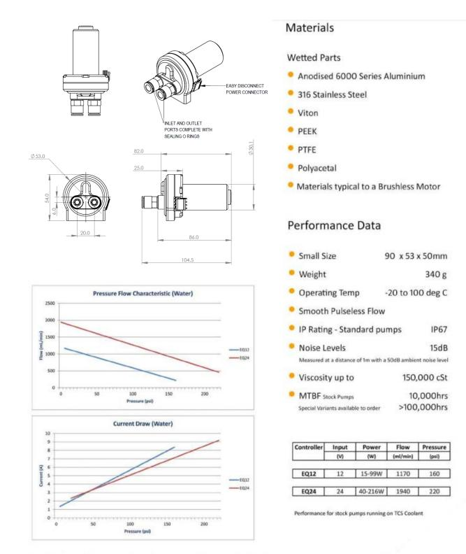
Pressure shown is the not to exceed value. All MG2000 pump variants are capable of more than the indicated figure but exceding this may result in damage to the pump.
