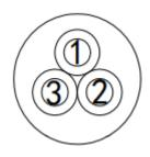
Cable Marking: RS PRO 3 Core×0.25mm<sup>2</sup> Unscreened Industrial Cable 250V
