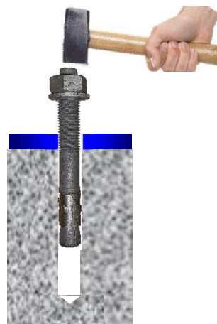
Insert assembled anchor through fixture into concrete
