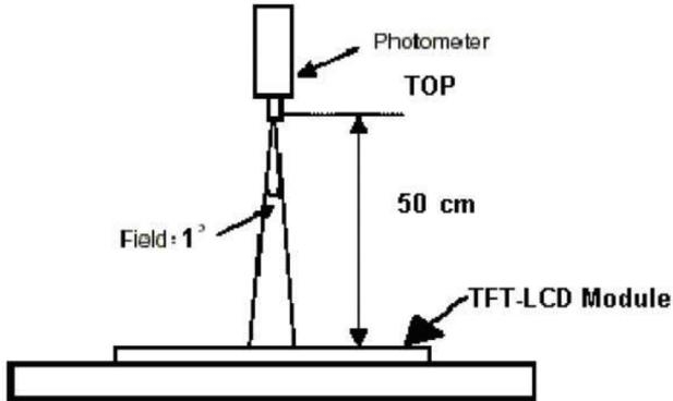
**Note 2:** Measured at the centre area of the panel and at the viewing angle of the  $\theta_x = \theta_y = 0^\circ$
