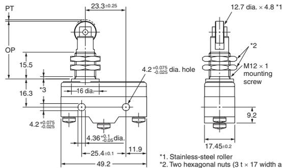
Note: Do not use the M12 mounting screw and the case mounting hole at the same time, or the case may be damaged.
