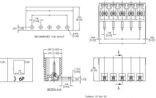
Positions: 02 thru 24 A= .138 [3.50] x No. of Spaces + .169 [4.30] B= .138 [3.50] x No. of Spaces
