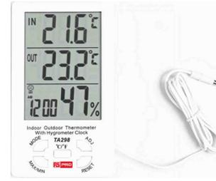
Accurate measurement of temperature and humidity, suitable for use both indoors and outdoors. The TA298 features a sleek and stylish design with a 66 × 92mm digital LCD display screen to simultaneously monitor indoor/outdoor temperature and humidity with ease, accompanied by a user-friendly interface allowing the settings and program to be adjusted with ease
