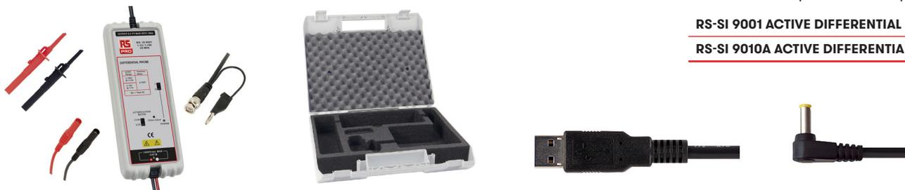
The RS-SI 9001 allows safe and accurate measurements between two voltage signals that are referenced to each other and has a switchable attenuation of 10:1 and 100:1, 25 MHz bandwidth and  $\pm 700$  V maximum differential. The probe can be operated either by 4xAA batteries or by the supplied USB power lead.
