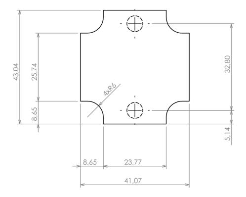
Dashed line shows outline of the mounting boss under PCB board Recommended mounting holes diameter ø3,5mm
