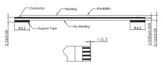
Dimensions: Millimetres Tolerances: ±0.3mm
