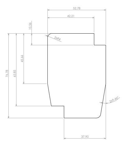
Dashed line shows outline of the mounting boss under PCB board Recommended mounting holes diameter ø3,5mm All dimensions are given within +/-0,5mm tolerance
