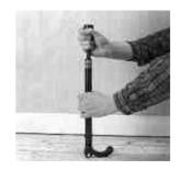
Position the Nail Puller over the nail to be removed
