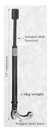
For easy removal of almost every type of nail even if sunk below the surface, simply sink the jaws in around the nail using the integral slide hammer. The heat treated alloy steel jaws act in the same way as a pair of pincers whilst the long handle givers excellent leverage.
