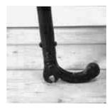
Lever the tool on to its curved foot to close the jaws in a firm grip
