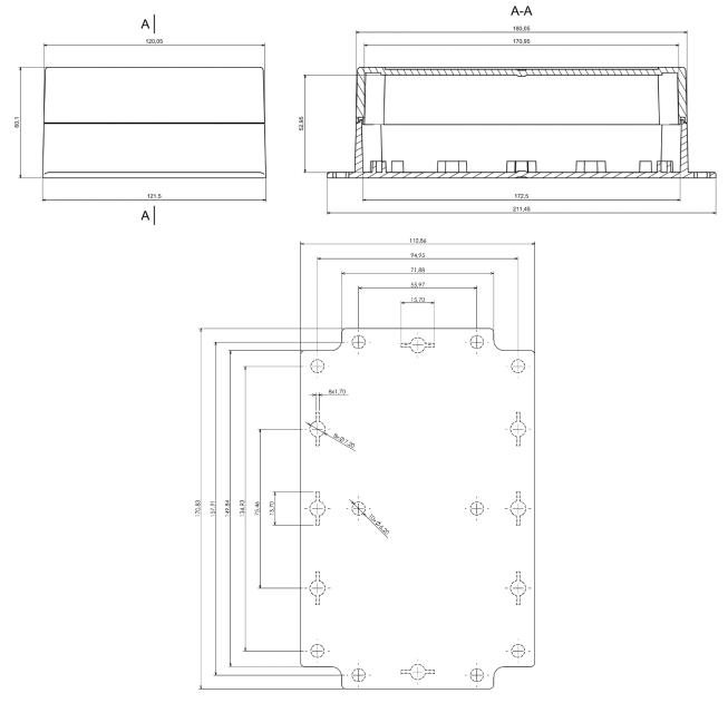
Dashed line shows outline of the mounting boss under PCB board Recommended mounting holes diameter ø4mm All dimensions are given within +/-0,5mm tolerance
