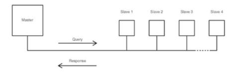
In the MODBUS Protocol the master can address individual slaves, or, using a special "Broadcast" address, can initiate a broadcast message to all slaves. The 236-9293 Digital meter do not support the broadcast address.
