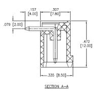
Positions: 02 thru 24 A = .197 [5.00] x No. of Positions+ .055 [1.40] B = .197 [5.00] x No. of Spaces
