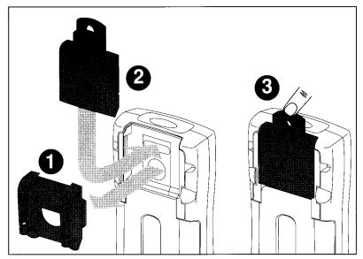
The LockPak accessory easily fits into the back of the meter, once the rubber probe holder is removed.
