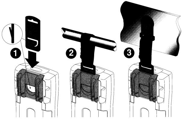
The universal hanger attaches to the meter and can be used by itself on a nail, hook, with a piece of rope or stiff wire.
