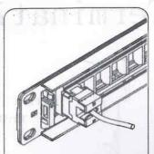
b. With the bottom latch engaged to the patch panel. rotate the jack upward until the flexing side of the keystone latch engages with the patch panel. There should be a slight clicking sound as the latch engages.
