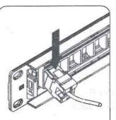
Insert the jack into its opening in the patch panel at an angle with the non-flexing side of the keystone latch facing down.
