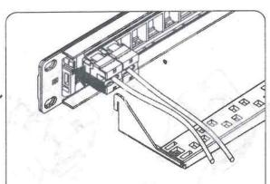
Align the tongue fo the wire minder with the corresponding groove on the patch panel and insert it into the groove.
