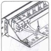
d. After installing two jacks, use a tie wrap to attach their wires to the wire manager. Do not over tighten the tie wrap! it should be snug. but not so tight that it crushes the wires. Continue this until all the jacks have been installed.
