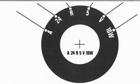
Aloxite "A" - Used for grinding and finishing all types of steel, except those sensitive to heat. It is the toughest of the aluminum oxide grains.
