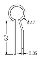
Hole in PCB  $\phi$ 0.8 to  $\phi$ 1
