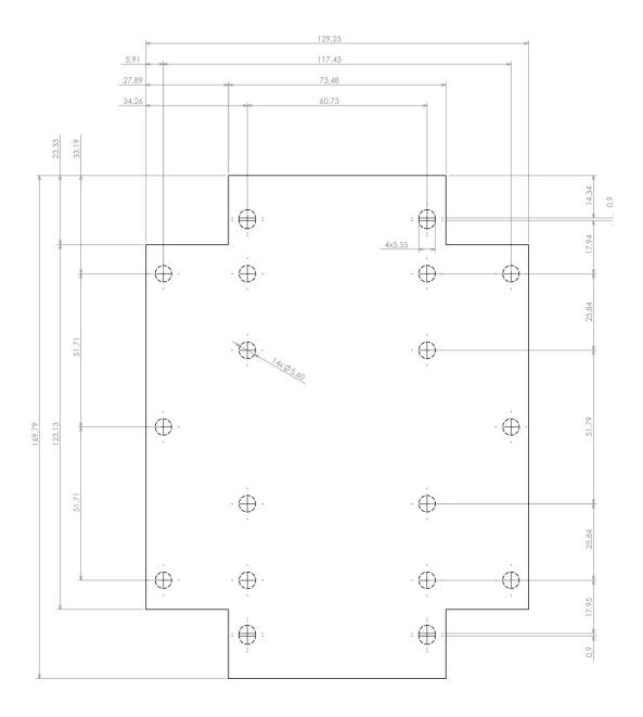
Dashed line shows outline of the mounting boss under PCB board Recommended mounting holes diameter ø4mm All dimensions are given within +/-0,5mm tolerance
