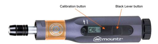
**Step 3:** The screen will briefly display "CAL" before showing the torque unit selection screen. Press Lever button to cycle through the options to reach your desired units, then press Calibration button again to select.
