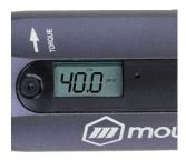
The value displayed when selecting the model is the max range of the tool and displays on whatever units were selected before. If you are calibrating an FGA-8 in cN.m, you need to choose the maximum capacity for that model in cN.m torque unit.
