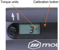
**Step 4:** Using the Lever button, cycle through the ranges until the display reads the value corresponding to your tool model. Then press the Calibration button to accept. A breakdown of the models and their display can be found below.
