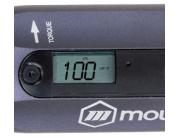
**Step 10:** When all set points are complete, the screen will flash 'don' to signify the calibration procedure is complete. Tool will resume normal function using the new calibration afterward.
