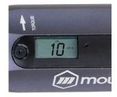
**Step 6:** Using the torque analyzer or sensor, adjust the tool to the target torque calculated based off of percentages of the max torque shown below. The tool must be set to the target value from a lower setting. If the target is exceeded, the tool must be adjusted below the target and readjusted up.
