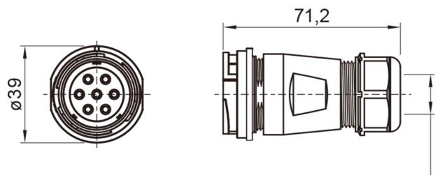
Cable outer diameter range: 13-16mm
