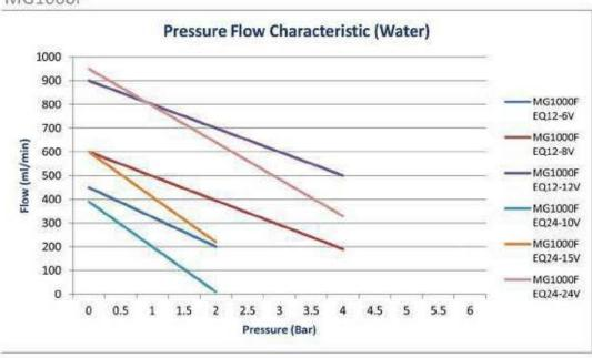
Pressure shown is the not to exceed value. All MG1000 pump variants are capable of more than the indicated figure but exceding this may result in damage to the pump.
