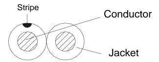
Cable Marking: RS PRO 2 Core×0.4mm<sup>2</sup> Speaker Cable 60V
