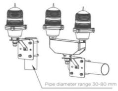
Ordering Code: AKU80 Mounting kit for 30-80mm vertical or horizonal pipe
