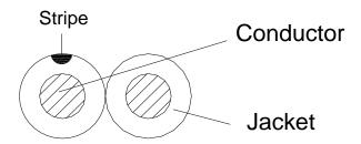
Cable Marking: RS PRO 2 Core × 0.34 mm<sup>2</sup> Speaker Cable 60V
