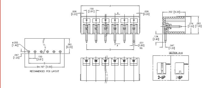
Positions: 02 thru 24 A= .150 [3.81] x No. of Spaces + .181 [4.60] B= .150 [3.81] x No. of Spaces
