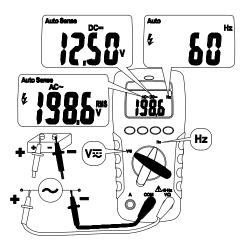
Dial the switch and press the Function button to select the measuring function.
