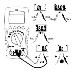
Dial the switch and press the Function button to select the measuring function.
