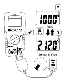
Dial the switch and press the Function button to select the measuring function. (°C / °F)
