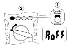
Dial the switch to off position ,then keep the Function button down and turn the meter on.
