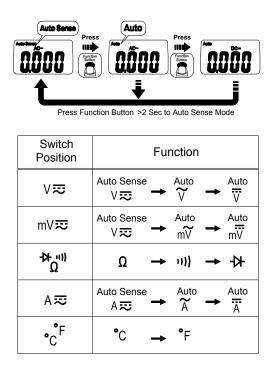
Press the Function button to change the function on the same switch position.
