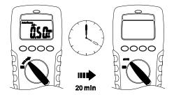
Wake-up the meter by dialing the switch or pressing any button.
