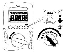
Dial the switch to off position ,then keep the HOLD button down and turn the meter on.
